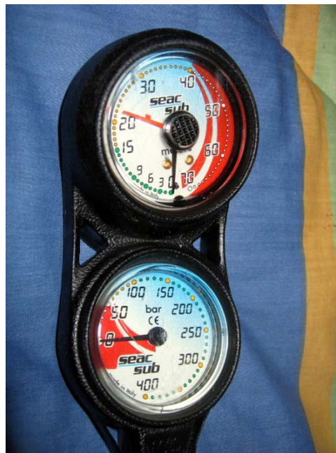
Fig A4.1. Dial-type diving gauges includes preset marker and colour-coded status zones, as well as indication of current reading
